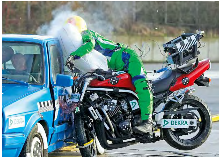
Considerable potential exists for increasing the safety of motorcyclists, too. Crash tests yield important findings here.
